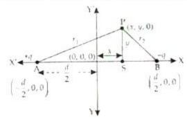
Then equipotential surface will pass through S and perpendicular to line joining two chargers or AB.
