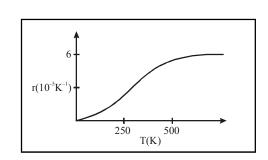
Coefficient of volume expansion of Cu as a function of temperature.
