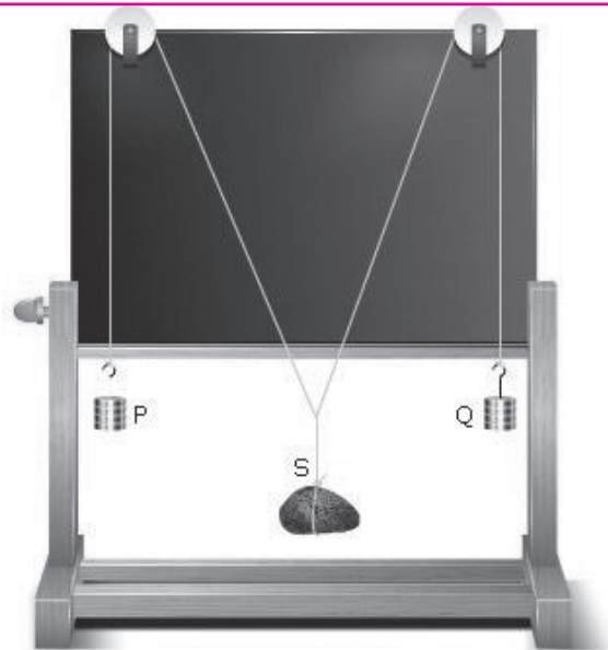
Fig. 4.2 Actual set up of parallelogram law of forces
