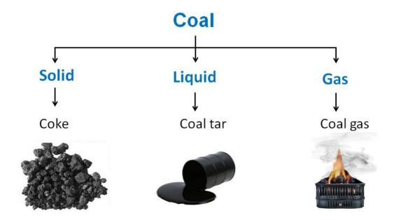
Coke: Coke is almost pure form of carbon, is tough, porous and black. Coke is used in manufacture of steel and extraction of many metals.
